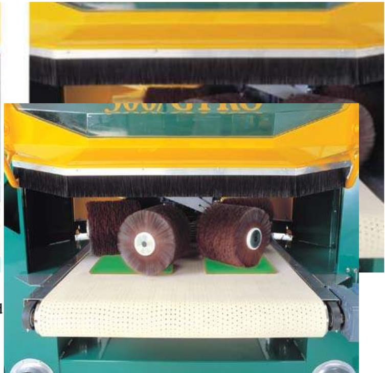
means that the processing of the surface is applied from every possible direction, no matter how the part is placed on the conveyor belt. This fact is especially important in set-ups where the machines are placed in a line, making it possible to utilise the full 1300 (GYRO-model) working width.
