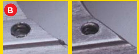
Before FLADDER® finishing. After FLADDER® finishing.
